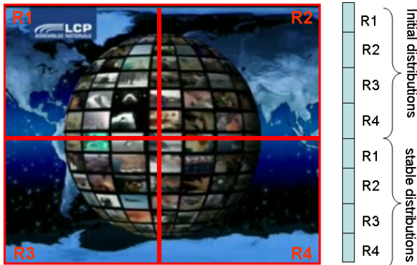
Figure 1. Extended MSF features. The left side shows the spatial division of a frame and the right side is the derived feature descriptor.
